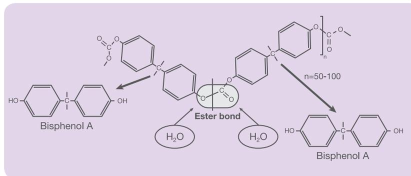
**Fig. 1** Polycarbonate is composed of molecules of bisphenol A linked by ester bonds. The ester bonds are susceptible to hydrolysis that increases as a function of temperature as well as an increase or decrease in pH relative to a pH of 7. Hydrolyzed BPA molecules are released into the surrounding medium.
